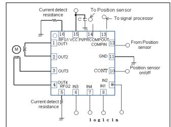
3. Example of applied circuit when connecting in parallel The use likened to H bridge 1ch is shown possible in the figure below by connecting IN1 with IN3, IN2 with IN4, OUT1 with OUT3, OUT2, and OUT4. (I<sub>O</sub> max = 0.8A, Upper and lower total  $R_{ON}$  = 1.35 $\Omega$ )
