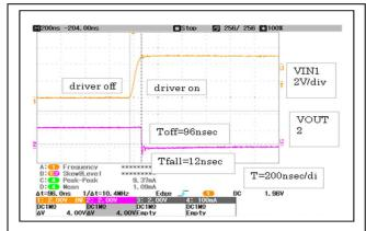
RFG-GND shorted load is 10kohm pullup & down (Fast decay)
