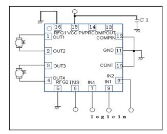
2. Example of applied circuit with one stepping motor driving
