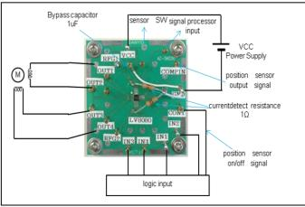
Connect a stepping motor with OUT1, OUT2, OUT3 and OUT4.
