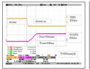
RFG-GND shorted load is 10kohm pullup & down (Fast decay)
